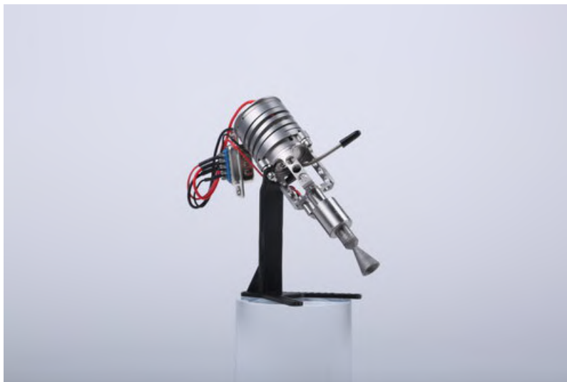
Figure 1.5: Busek BGT-X5 monopropellant thruster (sourced from [31]).
