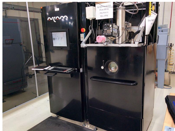
Figure 2. “Arcam A2” by William Sames, licenced under CC-BY-SA-4.0 [8].
