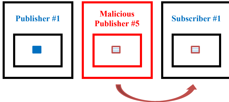
Figure 19: Self-contained Demonstration #5: Post-exploit state of DDS Entities (Host Hijacking)
