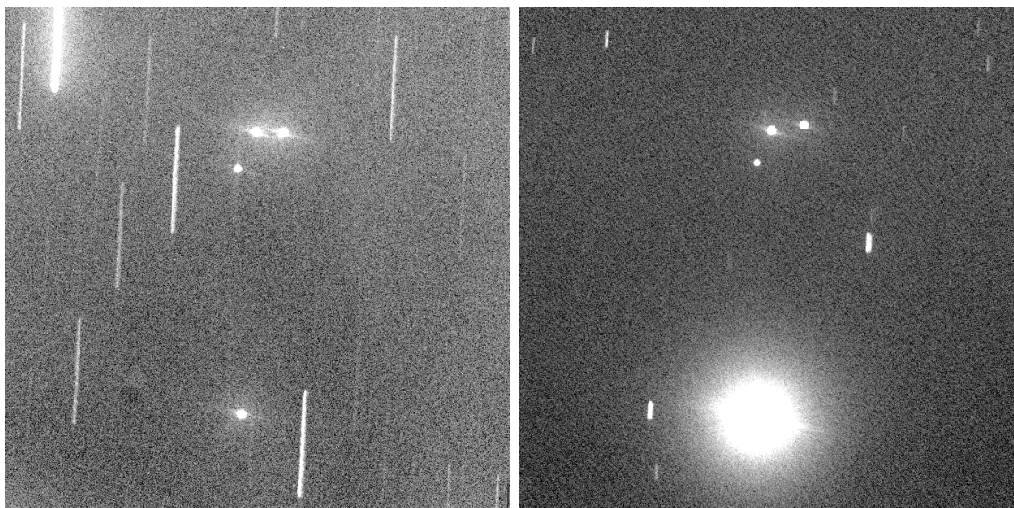
(a) Image showing all four satellites not saturating the CCD. (b) Image showing Echostar 17 (bottom of image) saturating the CCD.
