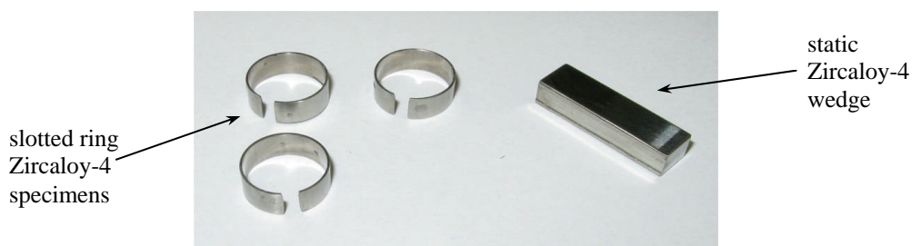
Figure 126: Zircaloy slotted rings and a static wedge prepared for I-SCC testing
