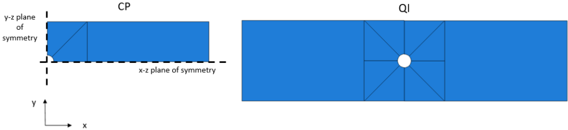
Figure 9: Geometry of Open Hole Tensile Test Specimen
